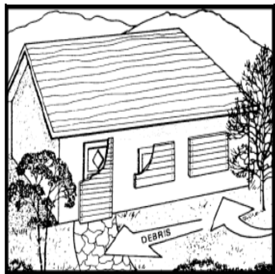
Figure 14. Using plywood to protect doors and windows 4
